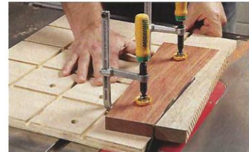
Add the dovetail clamps. These turned the sled into a ripping jig for straightening grain. Thanks to extra mounting holes for the miter bar, the sled can run with either its long or short side parallel to the blade.
