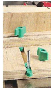
Handy hardware. The kit comes with a specialty bit for routing dovetail slots, four MatchFit clamp screws that slide neatly into those slots, and a ZeroPlay miter bar that attaches to the bottom of your shopmade sled.
