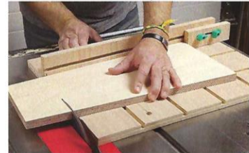
Free plan for a clever sled. The kit includes an excellent plan for a handy sled with criss-crossing slots that let you attach the fence in any direction. The fence includes a sliding stop.
