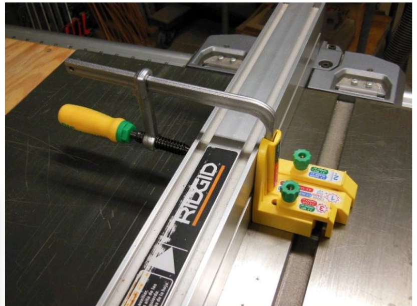
The included Matchfit Dovetail Clamp attaches the jig to your table saw fence (The clamp also has many other cool uses, some of which we'll cover at another time).
