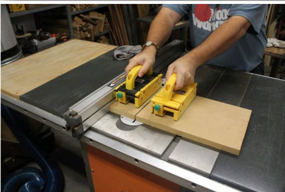
Calibration begins with a 4" wide strip of MDF. I've used my Micro Jig GR-RIPPER 3D Pushblocks for years now and have come to swear by them. (Be careful with long, narrow pieces that can twist and become wedged between the fence and blade. They can cause dangerous kickback.)
