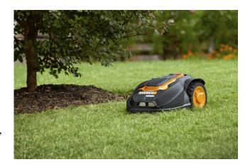
In fact, a robotic mower performs most effectively when used a few times a week, trimming a small amount each time. That way, the clippings are fine enough to sift back to the ground (instead of sitting on top of the grass to yellow in the sun.)
